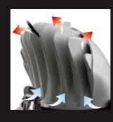
Multi wall construction heat sink
